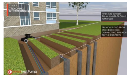
Figure 3.16 - Ground Source Heat Pump gathers heat from the ground via boreholes
