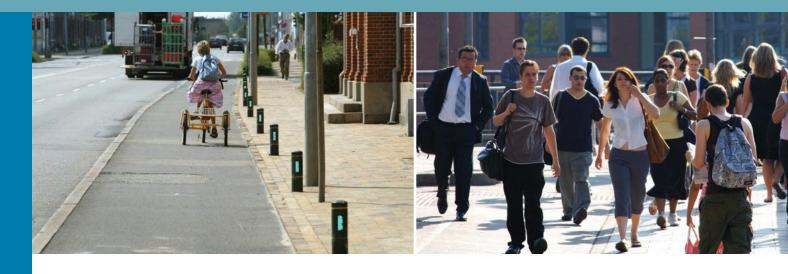
The Odense (Denmark) traffic management system (above left) rewards cyclists, and drivers who keep to cycling speed, with a regular green light at junctions, guided by the "green wave" of roadside LEDs
